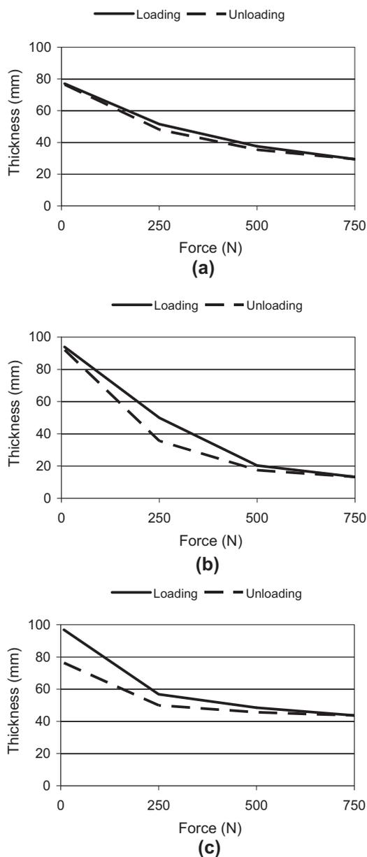
**Fig. 2.** Load deflection plots (a) 75 mm thick Sunmate soft cushion, (b) Propad, (c) Vicair Adjuster 10. Values are averages of three cycles as required by ISO 16840-2:2007.
