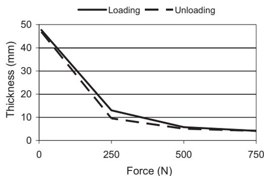
**Fig. 4.** Load deflection plot for 50 mm thick CM35 foam cushion. Values are averages of three cycles as required by ISO 16840-2:2007.
