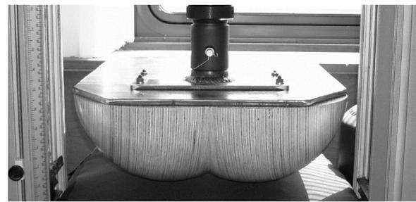
Fig. 1. Rigid cushion loading indenter (RCLI).
