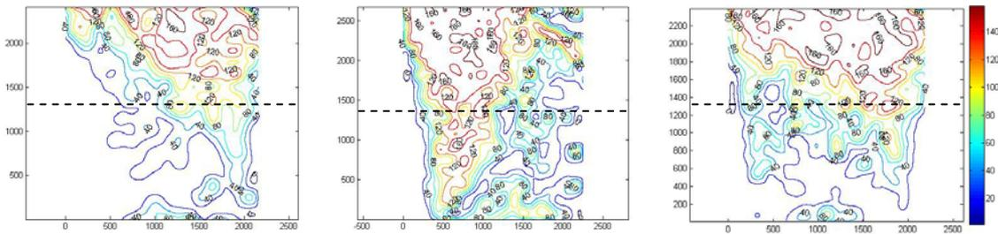
Figure 4: Foams irradiated at same frequency (20kHz) and variable distance from the maximum acoustic pressure: at 0cm, at 3.7cm and at 7.4cm. (Dashed line represents the irradiation plane for these samples)
