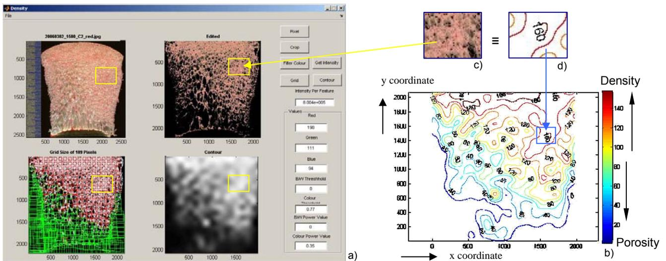
Figure 3: a) MatLab™ Interface; b) isoporosity contour lines; c and d) correspondent areas in image analysis and contour lines
