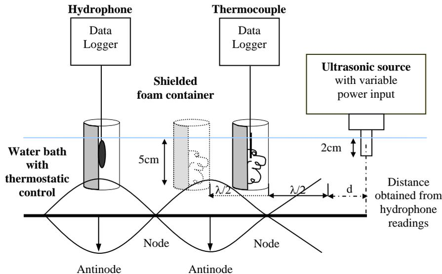
Figure 2: Schematic of the experimental rig with a representation of sonic field (mapped by hydrophone)
