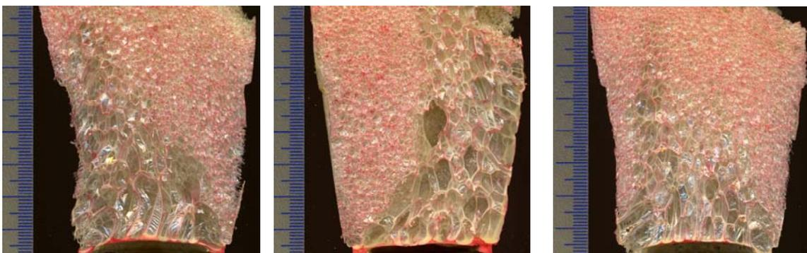
Figure 1: Cross-section of foams sonicated at different distances from the probe but same acoustic pressure (irradiating source was located on the left of these cross-sections)
