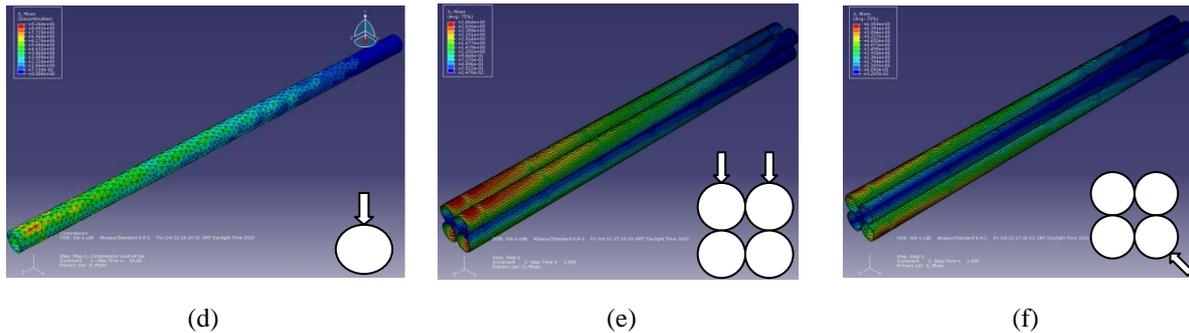
Figure 4: (a-c) Stress distributions when culms are under compression loading at top of the culm for the configurations: single culm, three culms in triangle formation, and four culms in zigzag formation; (d-f) stress distributions of different culms arrangements after variations in bending force parameters. The directions and positions of the forces are noted in the figures
