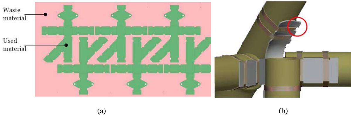
Figure 1: (a) Distribution of connection plates for stamping to minimise waste; (b) Model of the jointing approach. The strap is wound around the bamboo culm and the metal plate (circled)
