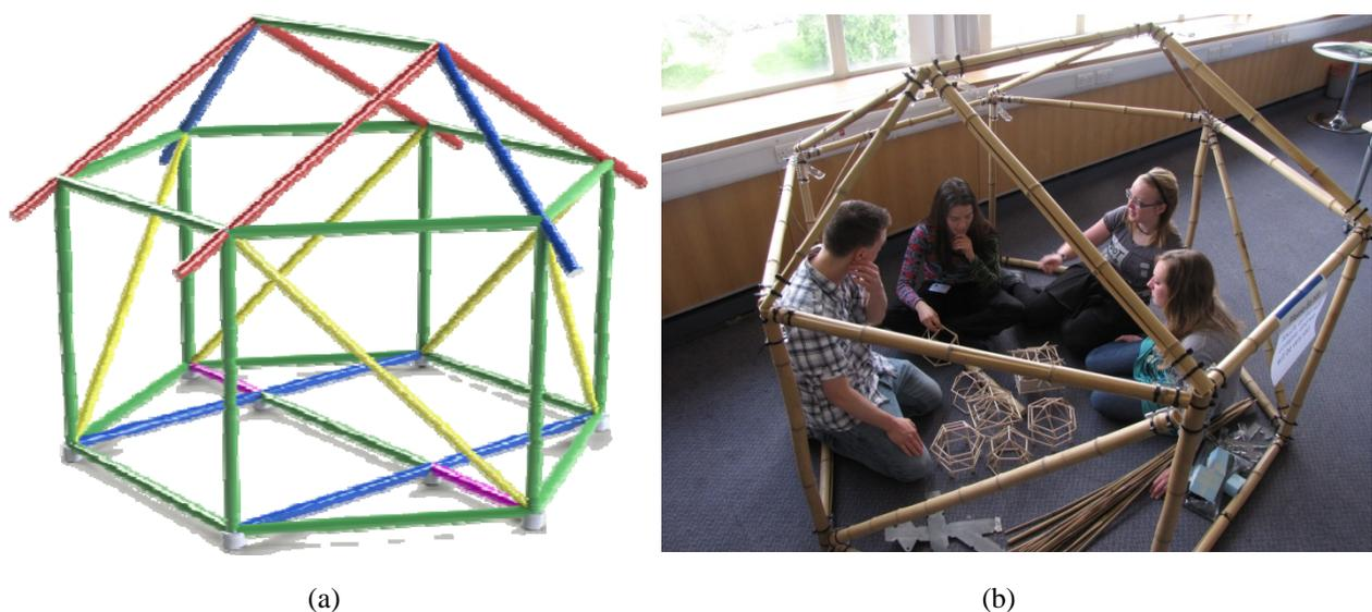
Figure 2: (a) Model of the bamboo hut, coloured scheme for the different parts; (b) 1:2 scale prototype built in Scotland being shown to EWB in June 2010
