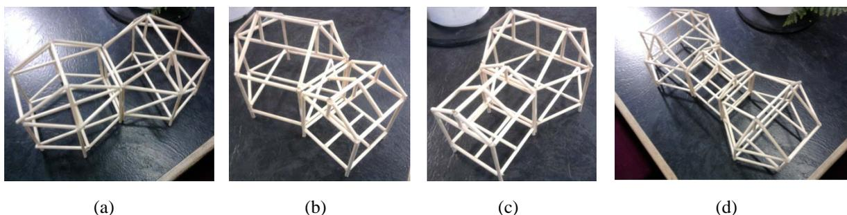
Figure 5: Spatial location of connected modules for an expanded bamboo hut structure
