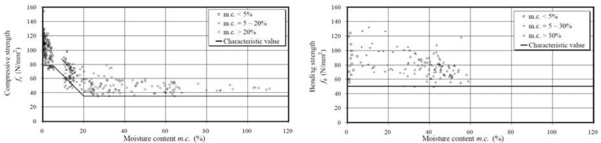
Figure 2: Compressive and bending strength vs moisture content in bamboo stems, as in [1]
